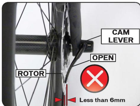
Fig. 1: Quick-release lever with potential for contact
